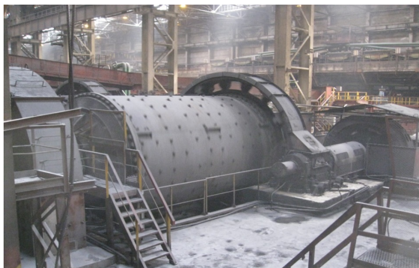
Figure 1 – Appearance of a ball drum mill
